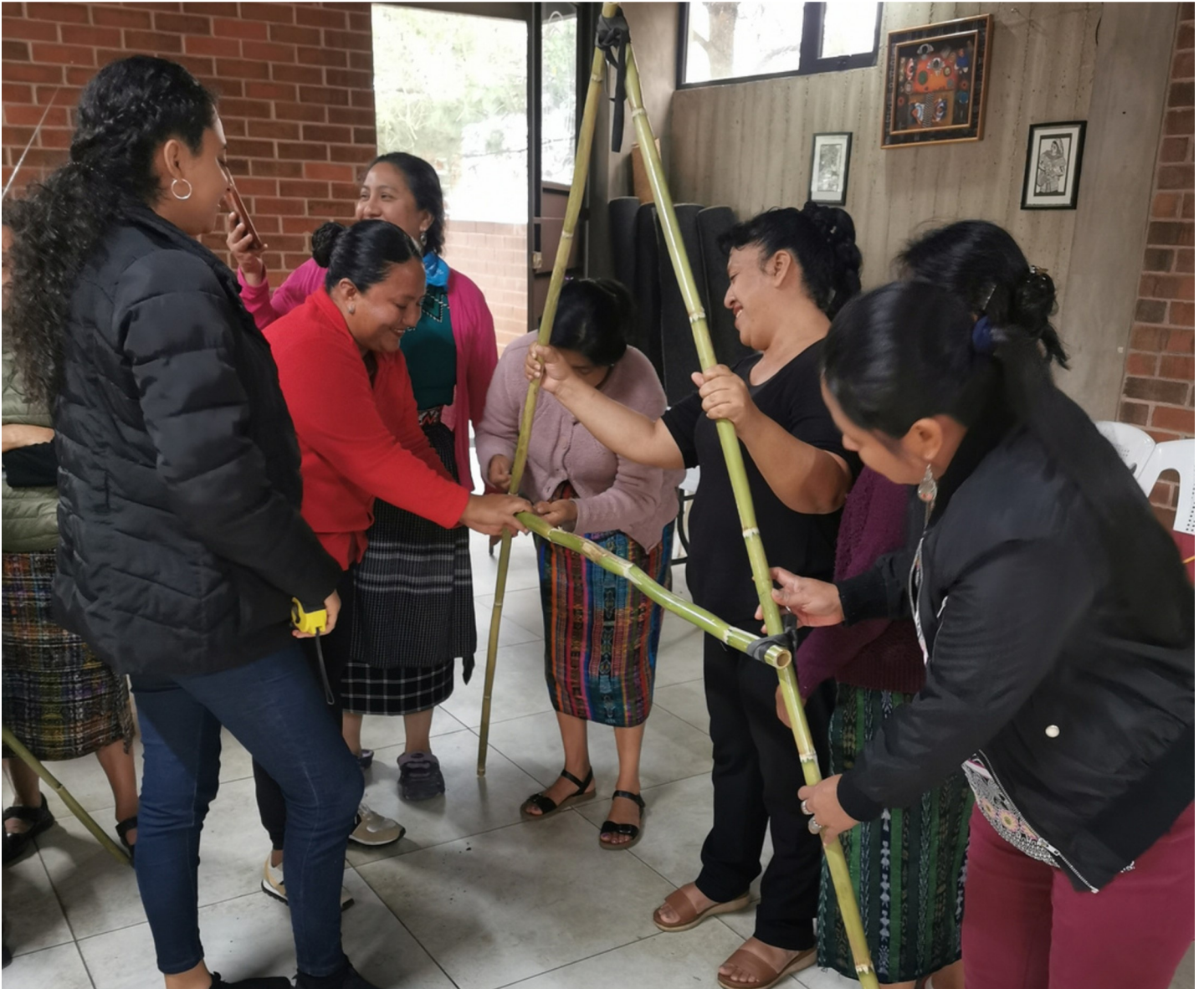
Development of Device A, designed for measuring soil levels, Permaculture Course, June 26, 2025. Kaqla Mayan Women's Center, Sacatepéquez
